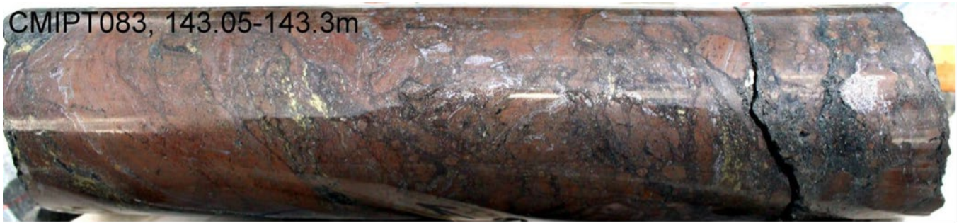
FIGURE 7: Core sample from Commonwealth Main area second massive sulphide unit in Hole CMIPT083: massive and brecciated massive sphalerite (red- brown) with lesser galena. Up to 3% chalcopyrite (yellow) is present in places. There is inherent uncertainty in reporting visual results which may only be confirmed through laboratory analysis. Refer to Appendix 3 of the Independent Geologist's Report in Schedule 3 for JORC Table 1 information.
