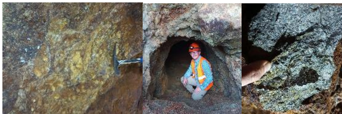
Figure 6.14 - Photos from within the open adit in western Laxia. From left to right: Disseminated sulphides / brecciated zone; opening to adit entrance, massive sulphide showing fresh mineralisation, in adit.
